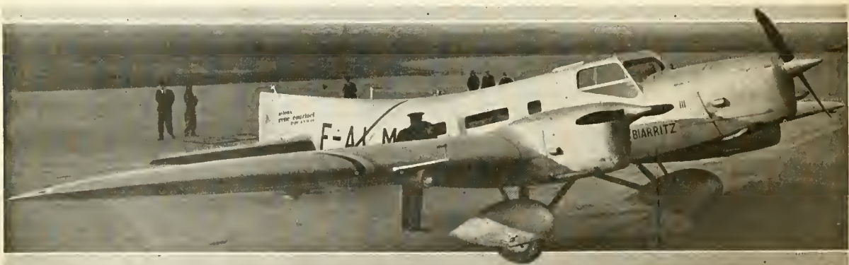
The French Couzinet 33 "Biarritz" powered with three 120 h.p. "Gipsy" inverted engines
